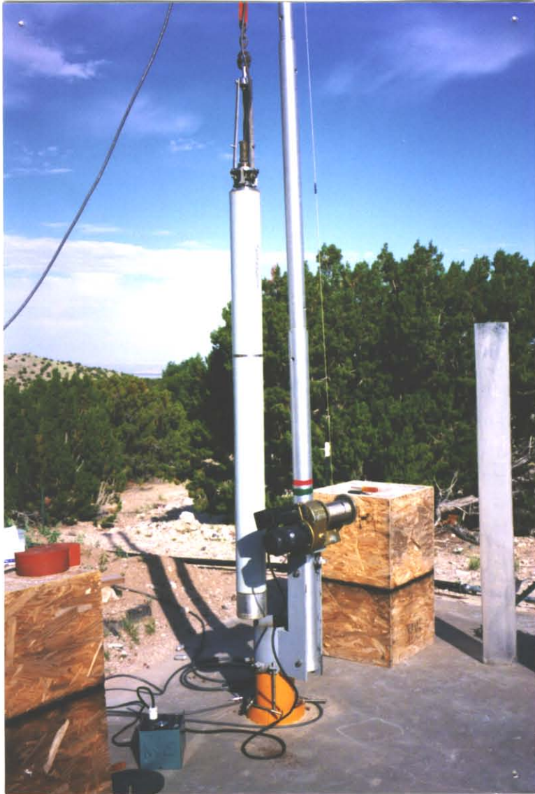
Entire KS-54000 assembly ready to be installed in sand in the borehole. Note the "sand foot" on the bottom of the sensor and the plastic borehole tube standing on the right.
