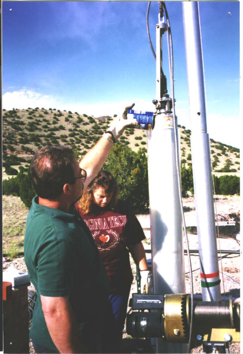
Pouring sand into a 6.5" ID transparent plastic borehole with a KS-54000 installed in the tube.
