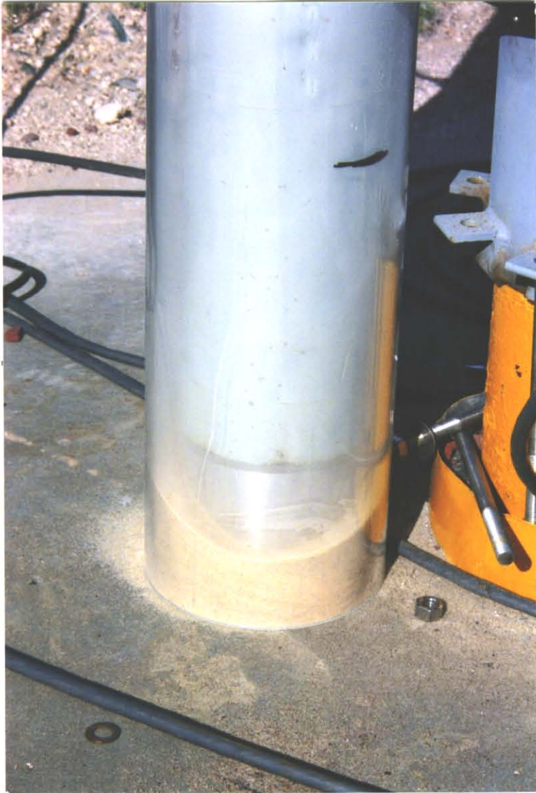
Sand accumulating at the bottom of the plastic borehole around the "sand foot".
