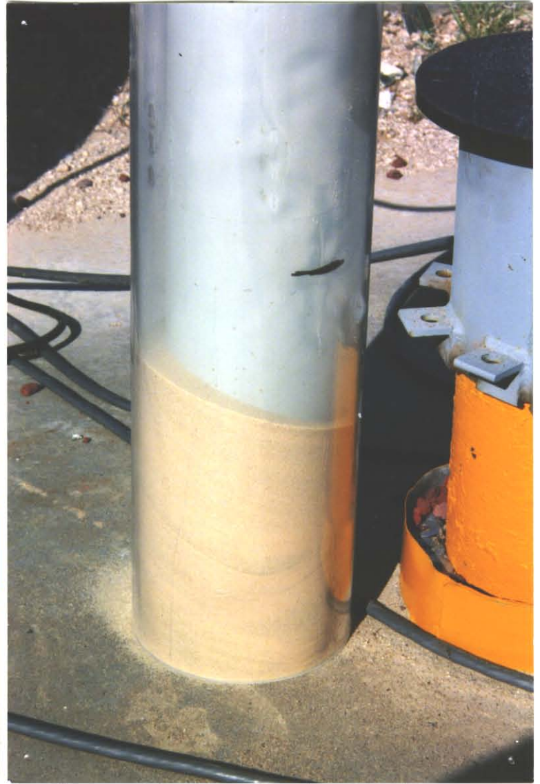
Sand accumulating in the annulus between the KS-54000 and the inner wall of the plastic borehole.
