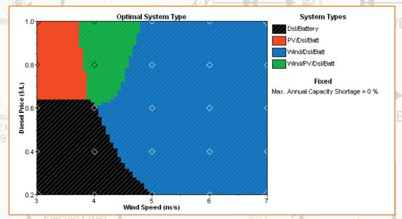
HOMER identifies the least-cost option under a variety of user-specified scenarios. For this off-grid analysis, it shows the minimum fuel price for PV to be cost-effective, the minimum windspeed for wind to be cost-effective, and the conditions under which a PV-wind hybrid are optimal.
