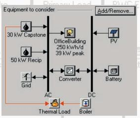
HOMER simulates all the hourly energy flows for complex hybrid systems. This schematic shows the variety of technical choices that HOMER optimized for a particular analysis.
