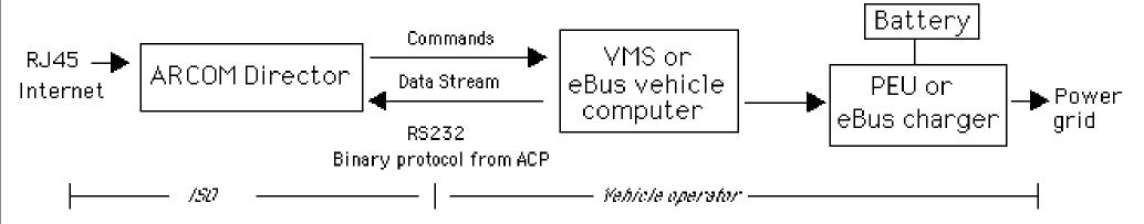
V2G Phase II: One ARCOM controller per aggregator
