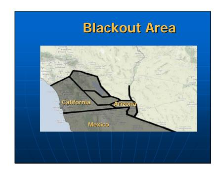
This slide shows the balancing authority/transmission operator areas affected by the blackout (and the islands into which they separated before the blackout).
