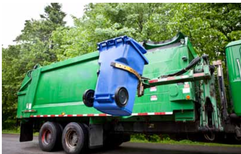
Municipal truck with robotic arm collecting residential waste for recycling. © Paul Vasarhelyi/iStock
