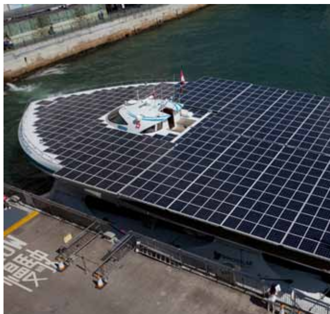
Tûranor PlanetSolar , the world's largest solar powered boat – topped by 500 m 3 of solar panels – was the first solar electric vehicle to circumnavigate the globe. © Tatiana Kakhill/iStock
