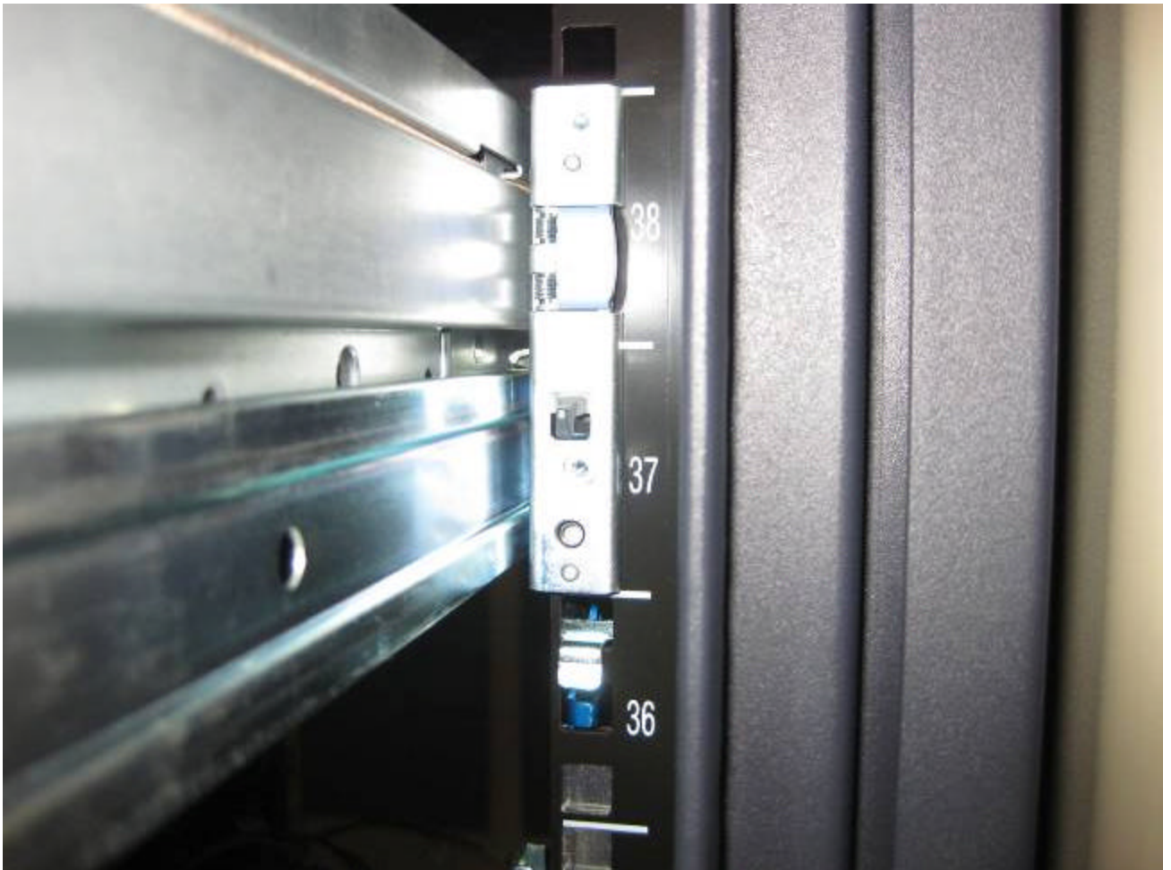
Figure A-2: Front Rail Flange for Dell R710
