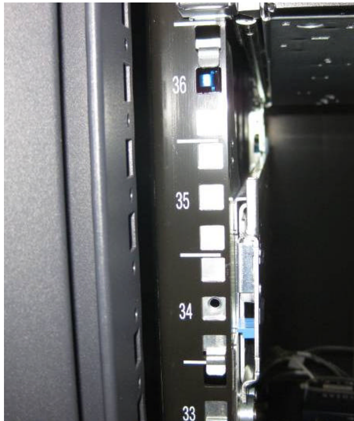
Figure A-5: R900 Rail Installed - Front of Rack
