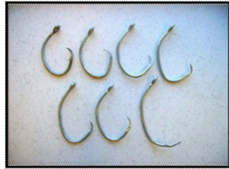
Hooks that retained bluefin tuna during the experiment: traditional hooks in the top row and weak hooks in the bottom.
