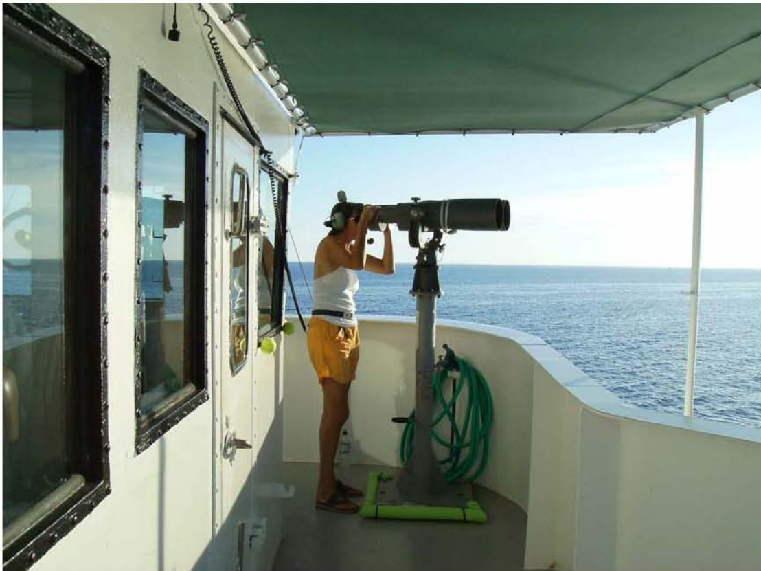
Figure 4-3. Big Eye binoculars and mount system on the bridge deck of the R/V Ranger.
