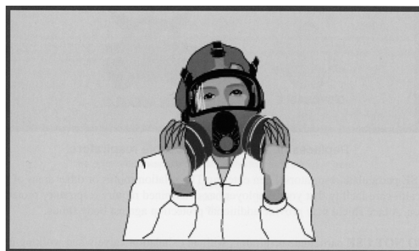
User Seal Check: worker covering inlet and inhaling (negative pressure check)
