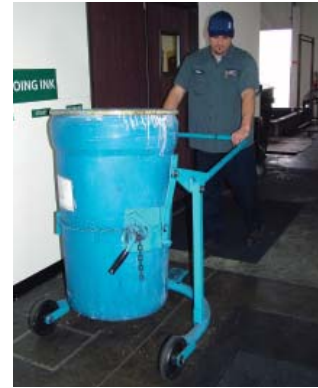
This drum dolly lifts and transports drums.
