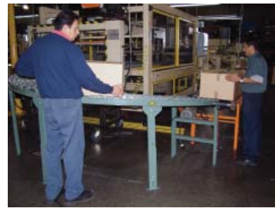
A curved skate-wheel conveyor moves containers around corners. It is activated by gravity.
