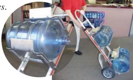
Two-wheel hand trucks work well for transporting bottles or cylinders over short distances.
