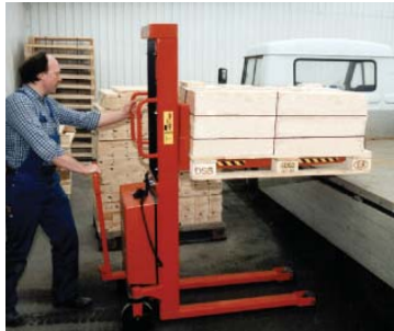
This stacker is well suited for moving loads up to 3,000 pounds for short distances.
