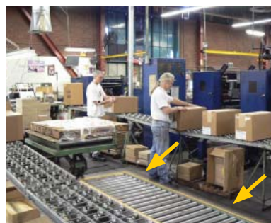
Floor-mounted roller conveyors can handle heavier pallet loads.
