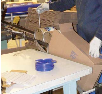
Design a conveyor system that delivers the container directly into position for loading.
