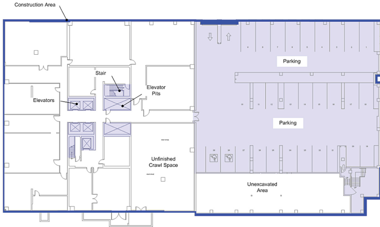
ILLUSTRATION 2.3-2: Basement floor plan with Structured Parking. Shaded spaces depict Unmarketable space.
