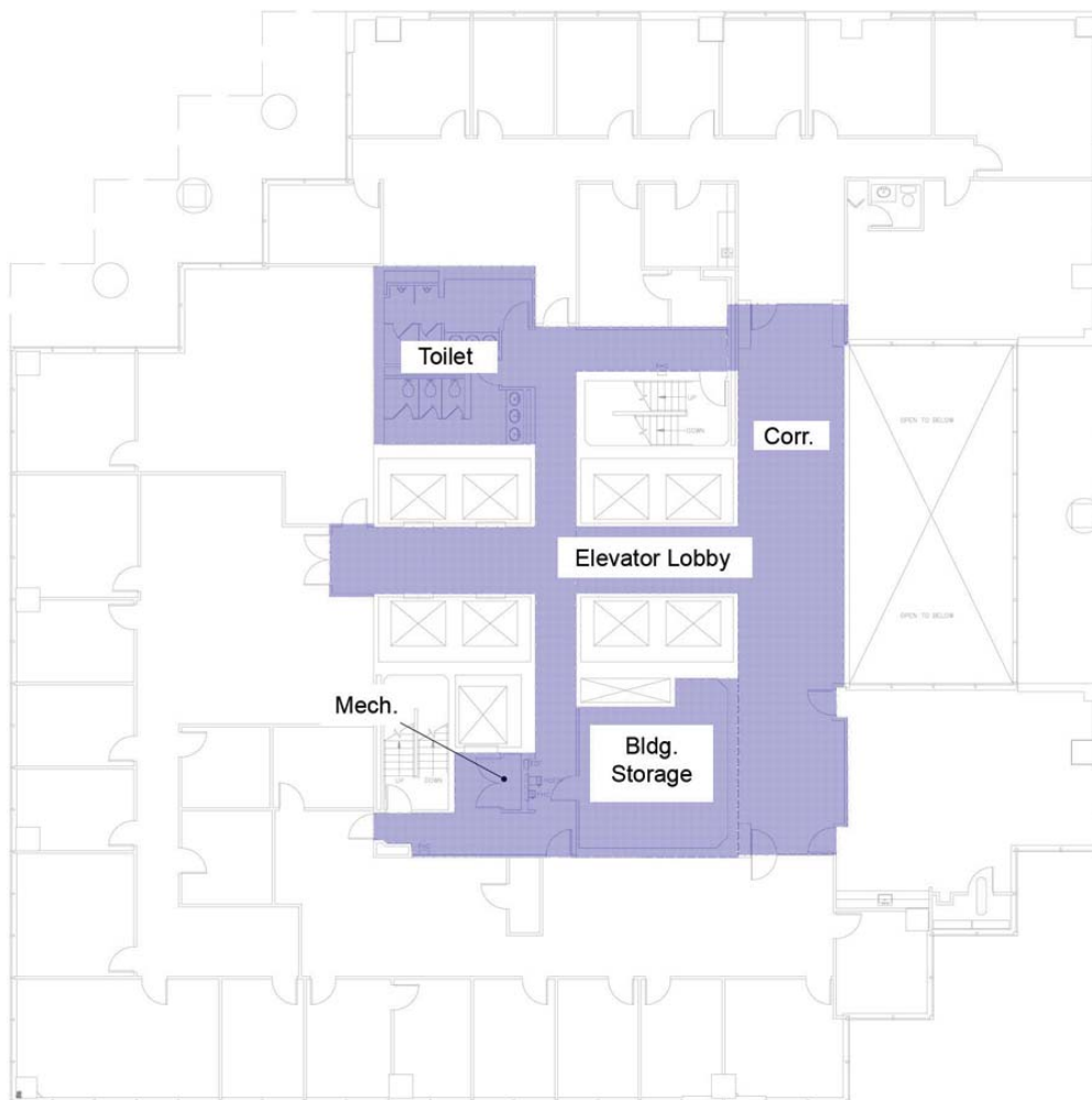
ILLUSTRATION 2.4-3: Shaded space depicts Common area of a floor plan.
