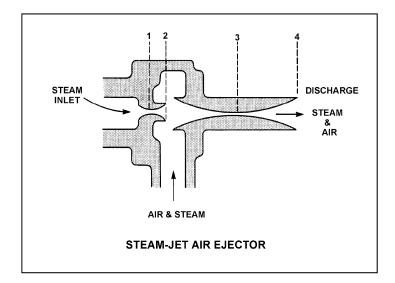
Refer to the drawing of a steam-jet air ejector (see figure below) in normal operation with steam reaching supersonic velocities.
