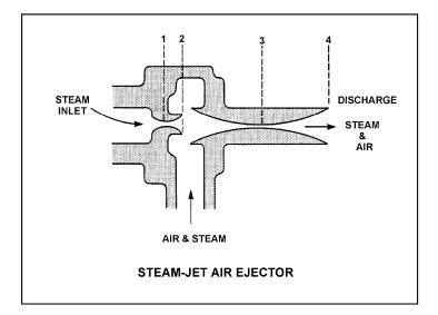
Refer to the drawing of a steam-jet air ejector (see figure below) in normal operation with the steam attaining supersonic velocity.
