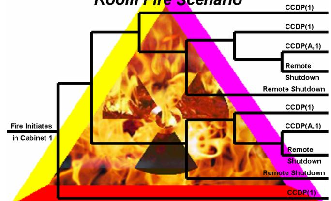
**Figure 1: Simplified fire event tree representing different sets of fire damage and plant response. The conditional core damage probability (CCDP) represents failure of only the cabinet in which the fire initiates, the additional fire-induced failure of train A, and fire-induced failure of both trains A and B leading to remote shutdown operations.**
