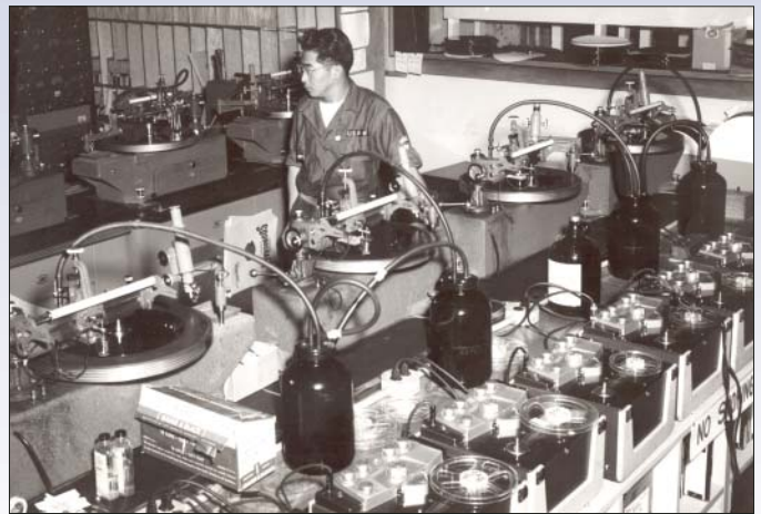
Army Language School media center transfers audio lessons from 78 RPM records to more durable reel-to-reel tapes.
