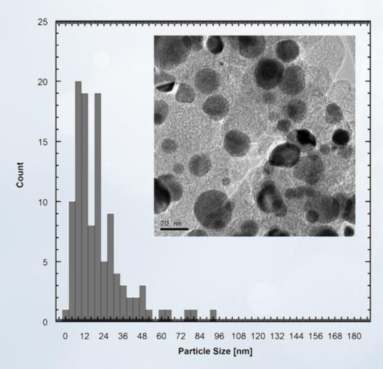
This TEM image shows Pd<sub>2</sub>Co nanoparticles having a mean diameter of about 12 nm. The size distribution shows that most of the particles have diameters less than 20 nm.
