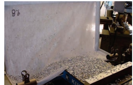
Chips collected by chip-catcher during dry machining
