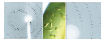
Figure 1. The x-ray diffraction patterns obtained from crystals of oxidized NAO. The diffraction pattern on the left was obtained with Cu K\alpha x-rays (1.54 Å), whereas the pattern on the right was collected with 1 Å synchrotron radiation. Synchrotron facilities provide a more intense, smaller, and focused x-ray beam. This enables longer crystal-to-film distances and the ability to resolve very closely spaced reflections from large unit cells.
