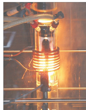
Figure 1. The radio-frequency furnace for endohedral fullerene synthesis in action.
