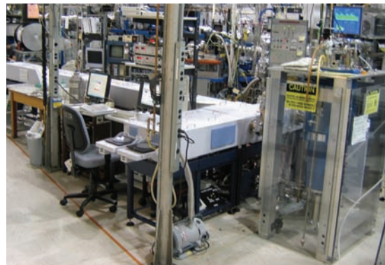
The Oxford Instruments magnet, installed next to the Bruker IFS 125HR spectrometer. The stainless steel tubes contain the optical coupling to the VUV-IR ring and between the spectrometer and the magnet.
