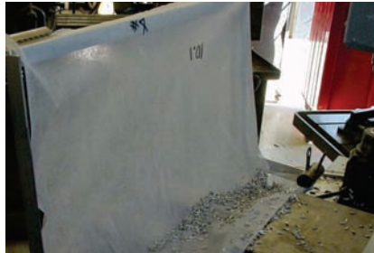
Chips collected by chip-catcher using vortex tube during machining
