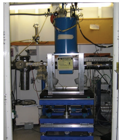
The magnet set up at X19A. It is mounted on a xyz table, which can be motor-controlled for ease of alignment. Samples are loaded from the top on a vertical rod into the samples space and are cooled by helium vapor or liquid from the magnet reservoir.
