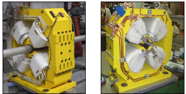
Figure 1: First article quadrupole magnets from BINP (left) and Tesla (right).
