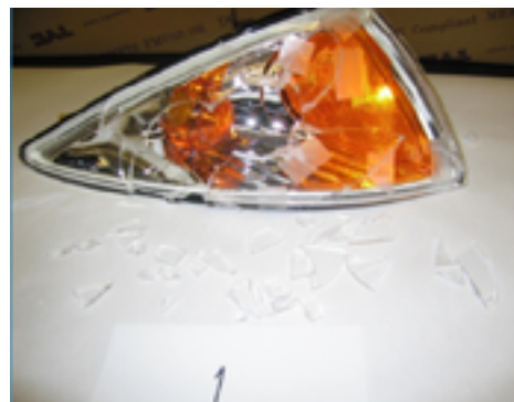
Figure 3. Assembly with major fragments physically attached.
