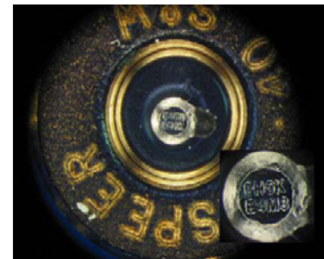
Figure 1. 40 caliber Smith and Weston cartridge case imprinted with the firing pin.
