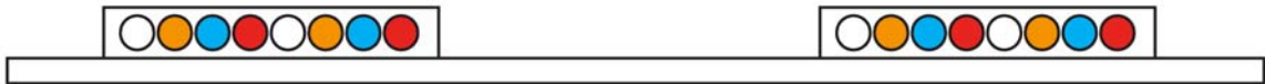
Figure 6. Schematic diagram of one of the experimental LED lamps, showing the layout of colors (white, yellow, blue, red) as viewed by a subject.
