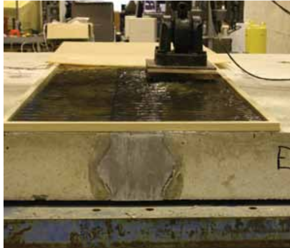
Ultra-high performance concrete connections are tested at FHWA's Turner-Fairbank Highway Research Center. These connections can link prefabricated bridge girders to precast concrete bridge decks.
