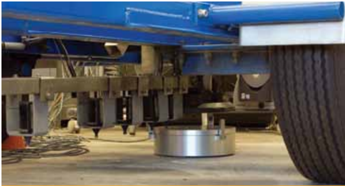
A falling weight deflectometer (FWD) is calibrated. Products and tools resulting from the Long-Term Pavement Performance program include a new FWD calibration system and an updated FWD calibration protocol.
