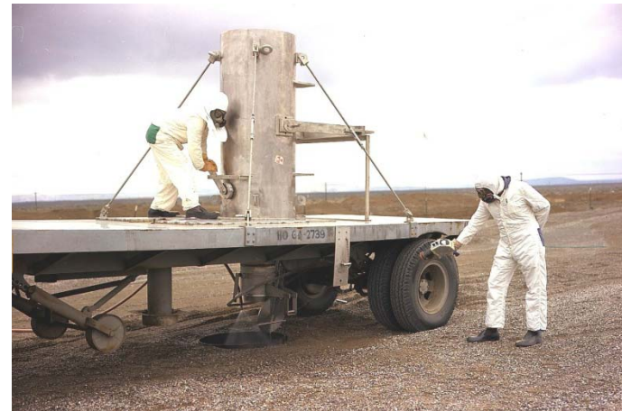
Workers dispose of waste into a vertical pipe unit.
