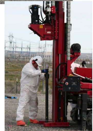
Two cone penetrometers were installed next to each vertical pipe unit.
