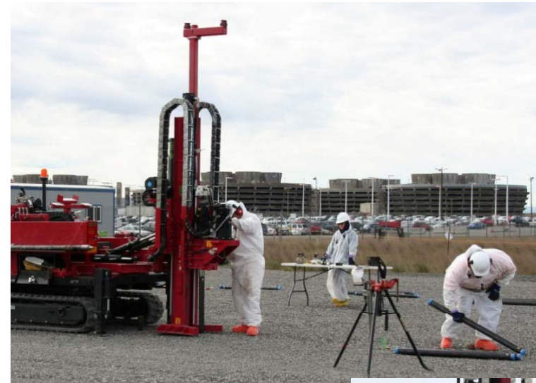
Two cone penetrometers were installed next to each vertical pipe unit.
