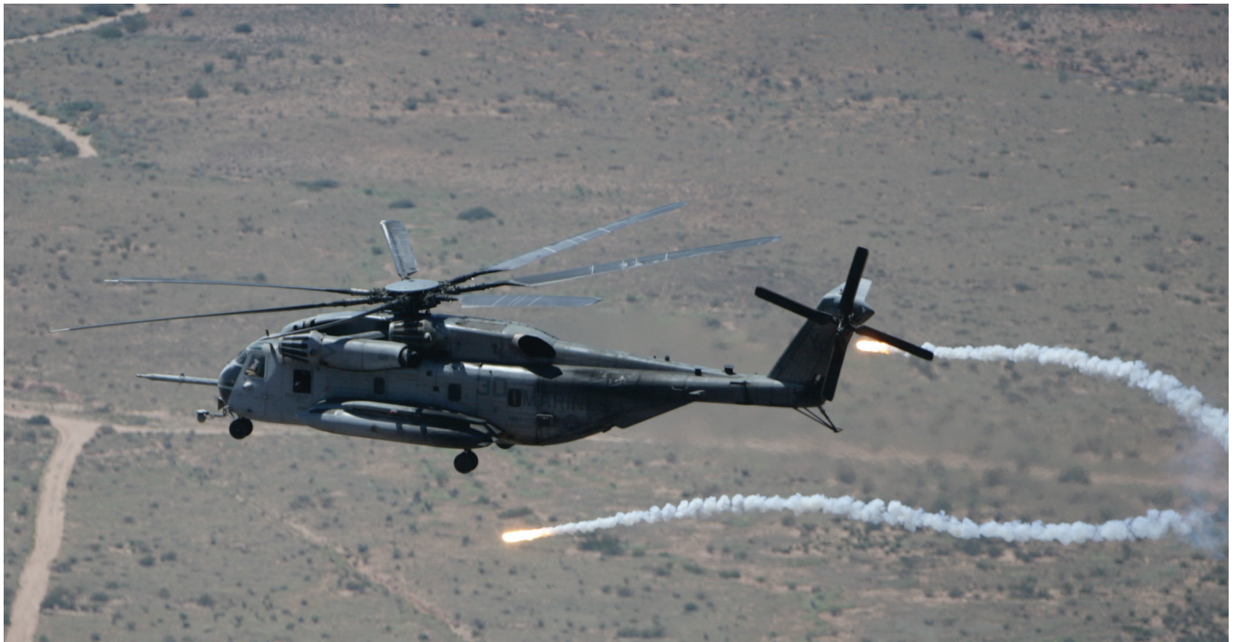
A U.S. Navy CH-53E Super Stallion tests the MJU-32A/B flare over the White Sands Missile Range.
