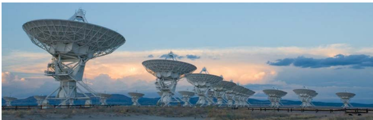
In FY 2013 the Karl G. Jansky Very Large Array (VLA) will begin full science operations. Transformed by upgrades in the hardware, electronics and computing of the existing VLA infrastructure, the Jansky VLA will provide order-of-magnitude improvements in observing sensitivity, spectral coverage, and resolution. Credit:NRAO/AUI
