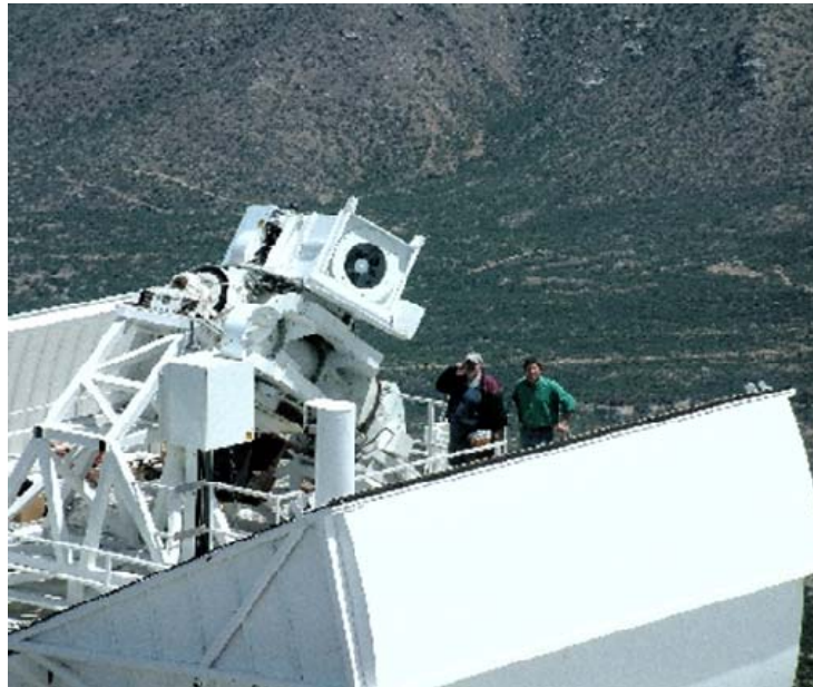
The NSO's SOLIS (Synoptic Optical Long-term Investigations of the Sun) instrument on Kitt Peak, Arizona. SOLIS provides detailed image, spectral, and magnetic data of the sun that is distributed in near real-time by the web. Credit: NSO/AURA.
