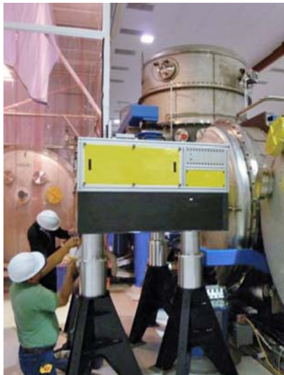
Installation of a quantum-mechanical squeezing experiment at LIGO in 2011. The temporary experiment allowed LIGO to increase its sensitivity by more than 20% over most of its frequency range. Such research is conducted by LIGO Laboratory and the LIGO Scientific Collaboration to reduce risk in the Advanced LIGO construction project. Credit: Caltech/MIT LIGO Laboratory.
