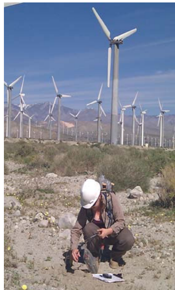
A student volunteer prepares to deploy a sensor on a wind farm near Palm Springs, California, that will record high-frequency seismic waves for the Salton Sea Imaging Project. Principal Investigators: John Hole, Virginia Tech, Joann Stock, Caltech, and Gary Fuis, USGS. Credit: IRIS.
