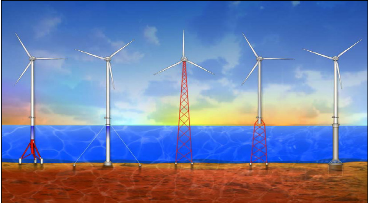
Figure 12.6 Example offshore wind turbine foundation types for transitional depths, 30-90 m (Robinson and Musial 2006).
