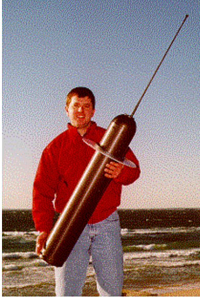
Fig. 1. Picture of a PALACE float. The PALACE float is 104 cm long excluding the 70-cm antenna. Its diameter is 17 cm and it weighs 23 kg.
