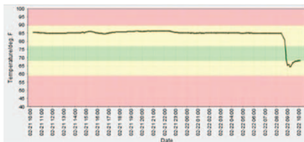
Figure 16. Effect of adding blanking panel to rack of high-performance servers.
