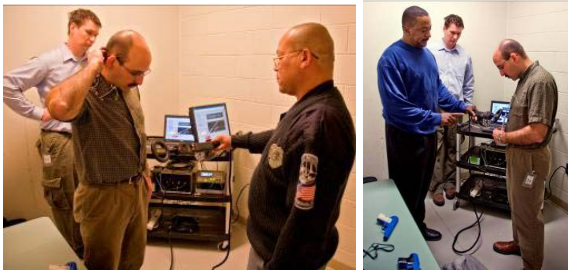
Figure 31: Photographs of the WANDD proof-of-concept device during testing at the Virginia Peninsula Regional Jail (VPRJ). Note the cart is used to house all of the electronic components along with the control laptop. The handheld device connects to all necessary electronics through a single cable bundle.
