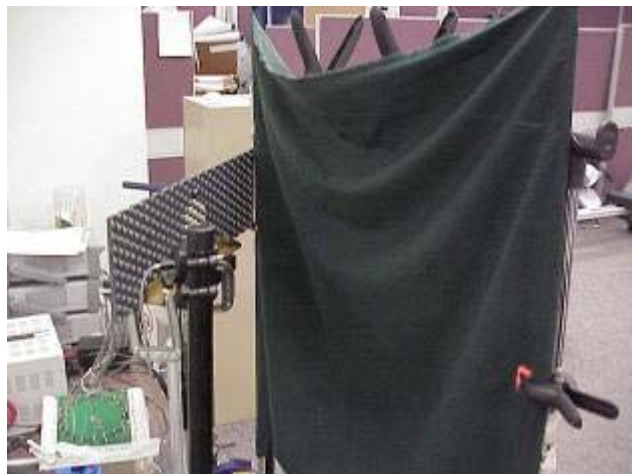
Figure 21: Photograph showing the wrinkled fabric used to test more “natural” fabric states that would be encountered in more practical applications. Compare this with the configuration shown in figure 18. The results of the tests under this configuration are shown in figure 22.
