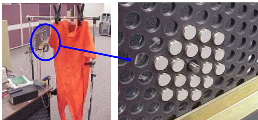
Figure 23: Photograph of the current configuration including: increased incidence angle, incorporation of microphone (silver) with the transmitters (white) and the inclusion of a standard VPRJ prison jumpsuit.
