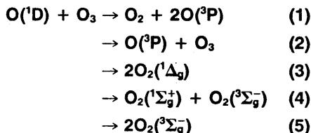
$$\begin{aligned} \Delta H''(1) &= -83.2 \text{ kJ}\cdot\text{mol}^{-1} \\ \Delta H''(2) &= -189.7 \text{ kJ}\cdot\text{mol}^{-1} \\ \Delta H''(3) &= -393.0 \text{ kJ}\cdot\text{mol}^{-1} \\ \Delta H''(4) &= -424.7 \text{ kJ}\cdot\text{mol}^{-1} \\ \Delta H''(5) &= -581.6 \text{ kJ}\cdot\text{mol}^{-1} \end{aligned}$$
