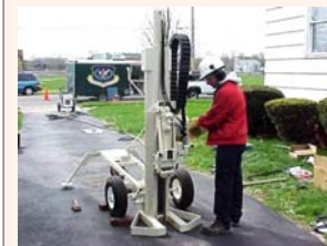
Fig. 6. Example of direct push technology for capturing soil and groundwater data.
