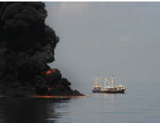
GULF OF MEXICO – Two fishing vessels drag an oil boom after trapped oil is set ablaze in the Gulf of Mexico as part of a controlled burn to aid in preventing the spread of oil. Photo courtesy of U.S. Navy
