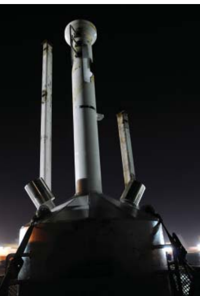
GULF OF MEXICO – A small pollution containment chamber, known as a “top hat” was used in an attempt to contain an oil spill caused by the Deepwater Horizon explosion. Photo courtesy of U.S. Coast Guard
