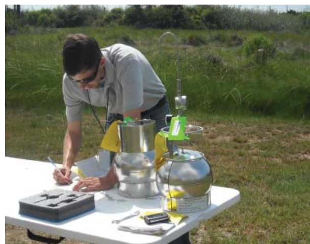
GRAND ISLE, La. – An Environmental Protection Agency contractor makes notations in log book as an air sampling instrument is replaced after a 24-hour cycle. Photo courtesy of EPA
