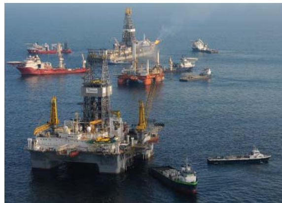
GULF OF MEXICO – The mobile offshore drilling unit Development Driller III (near) prepared to drill a relief well at the Deepwater Horizon site, as the MODU Q4000 held position directly over the damaged blowout preventer while making preparations for a “junk shot” or a “top kill.” The drillship Discover Enterprise (far) continued to capture oil from the ruptured riser. Photo courtesy of U.S. Coast Guard
