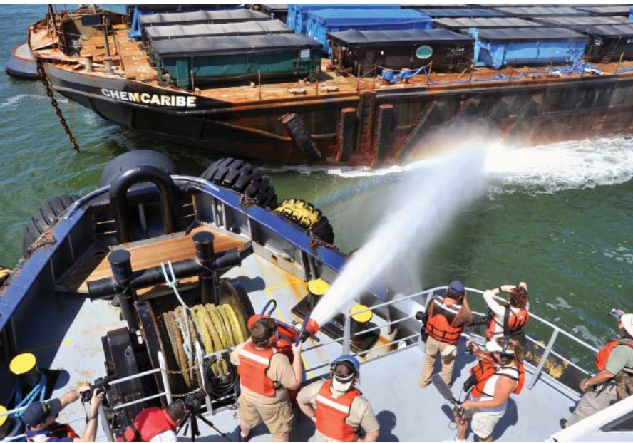
GULF OF MEXICO – A crewmember aboard a tug uses a high-pressure fire hose to wash oil from the hull of a barge as part of a gross-vessel decontamination process. Photo courtesy of U.S. Coast Guard
