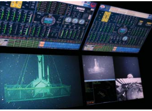
GULF OF MEXICO – Video acquired by a remotely operated vehicle is monitored and recorded. The video display shows a small pollution containment chamber, known as the “top hat” being lowered into the Gulf of Mexico. Photo courtesy of U.S. Coast Guard
