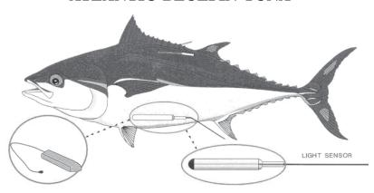
What are archival tags? Archival tags are electronic data-logging devices that provide location estimates by measuring light intensity through a light sensor. They also provide data on swimming depth, water temperature, and body temperature of the fish. This information is collected on a daily basis and stored in the tag for several years.
