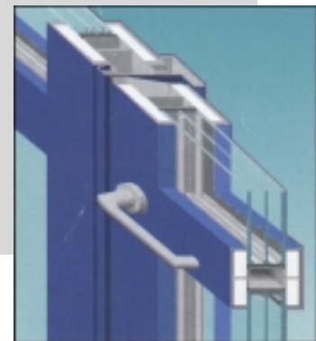
Fig. 13: Superlite II 90 minute laminated gel glass in steel door. (Section detail: O'Keefe)
