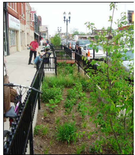
Rain gardens in Lansing MI clean stormwater and improve the streetscape (H.B. Rue).
