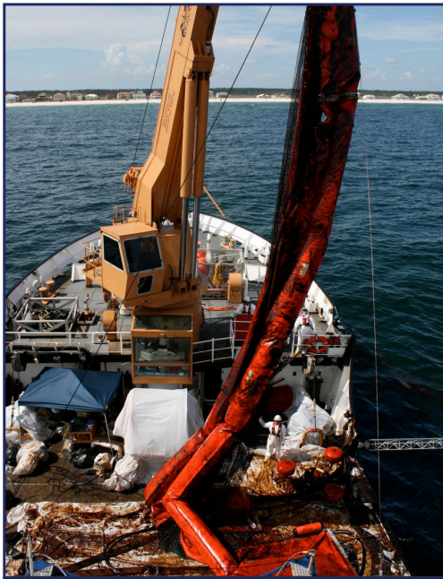
U.S. Coast Guard Seagoing Buoy Tender Aspen, homeported in San Francisco, recovers fast sweep boom June 28 after oil skimming operations in the Gulf of Mexico less than one mile from the shoreline. The Aspen is one of several Coast Guard vessels skimming oil in the Gulf of Mexico as part of the ongoing effort to combat the Deepwater Horizon oil spill. U.S. Coast Guard photo by Ensign Shea Winterberger
