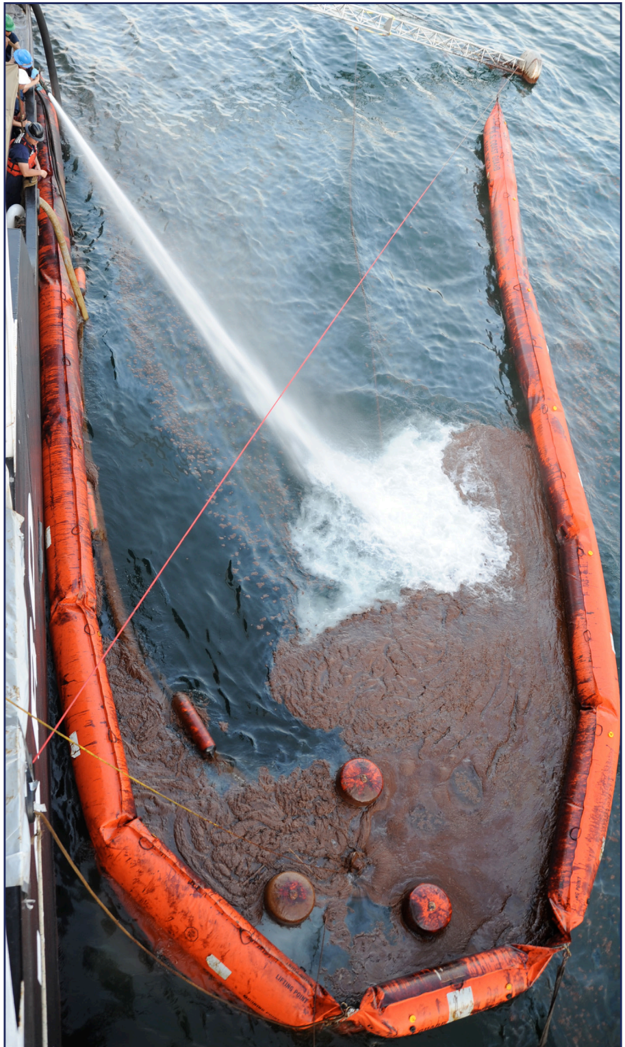
The crew of U.S. Coast Guard Seagoing Buoy Tender Juniper use the on-board fire hose from the buoy deck June 13 to direct surface oil collected into the Shipboard Oil-Recovery System pump. Crewmembers of the 225-foot Juniper, homeported in Newport, R.I., are conducting oil-skimming operations off the Alabama and Florida coasts in addition to the crews of Juniper-class seagoing buoy tenders Oak, Cypress and Elm. U.S. Coast Guard photo by Petty Officer 3rd Class Colin White
