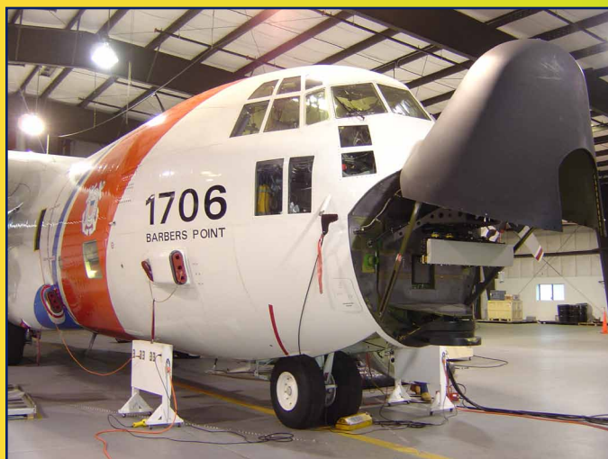
All of the Coast Guard's HC-130Hs now have their surface search radars installed. U.S. Coast Guard photo.
