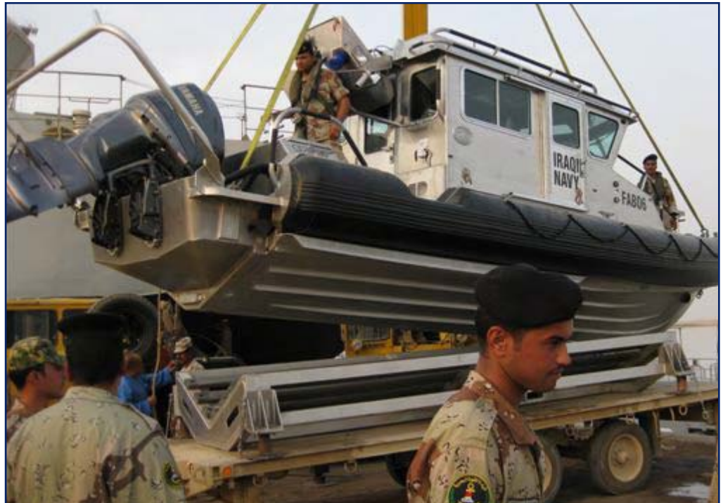
UMM QASR, IRAQ, Oct. 17—The Iraqi Navy's first Defender-class 25-foot response boats arrive at the country's principal naval base. In preparation for the boats' arrival, the Iraqis made a number of infrastructure improvements, including modified flatbed trailers that are mated to the boats' transport cradles. U.S. Coast Guard photo
