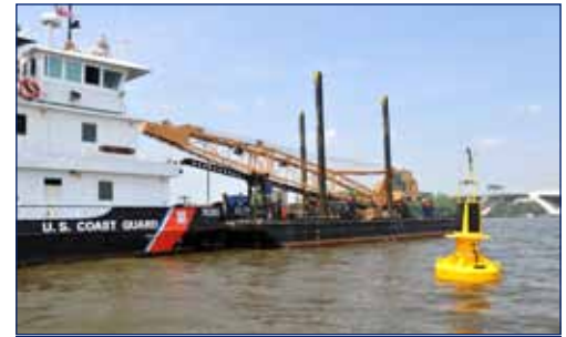
The Coast Guard Cutter Sledge is a 75-foot inland construction tender (WLIC) homeported in Baltimore. The average age of the WLIC class of tenders is 45 years old. The Coast Guard is looking into design alternatives to recapitalize these venerable work boats. U.S. Coast Guard photo by Petty Officer 3rd Class Robert Brazzell
