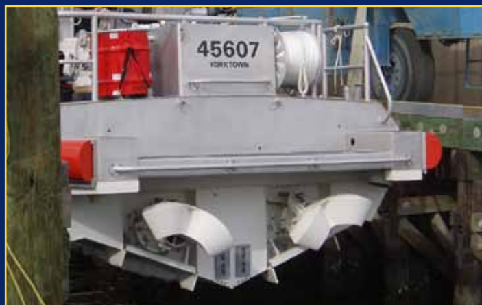
The RB-M's water jet propulsion system gives the boat its speed and maneuverability. U.S. Coast Guard photo
