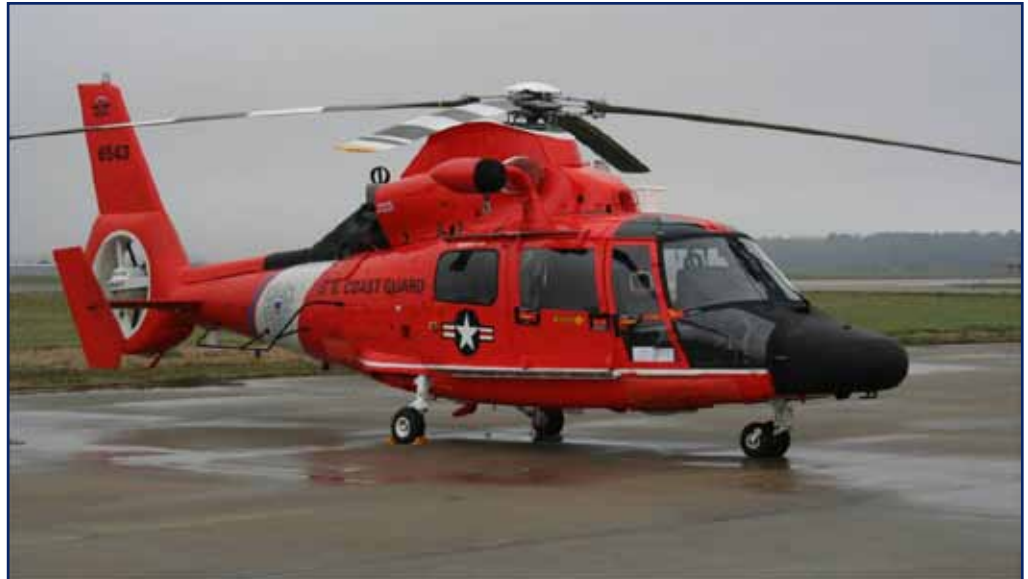
The Coast Guard has begun upgrading its MH-65C helicopters to MH-65Ds by adding digital components that are smaller and lighter than the old equipment, making the MH-65Ds more fuel efficient. U.S. Coast Guard photo
