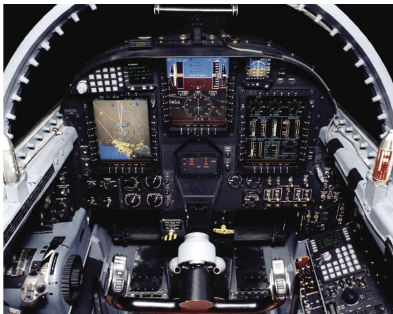
In the cockpit of upgraded U-2 reconnaissance plane
