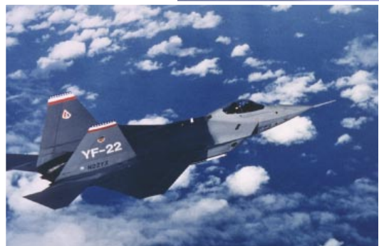
Flight testing YF-22 prototype.
