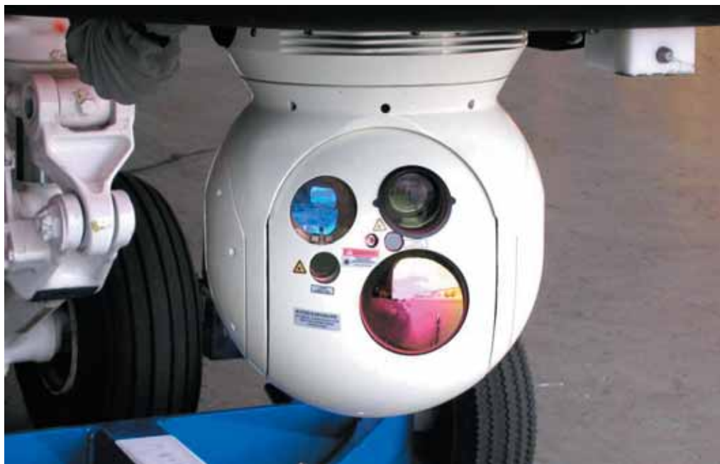
The MH-60T's new electro-optical forward-looking infrared turret is equipped with cameras, a laser range finder and thermal imaging sensors to improve aircrew situational awareness in day and night operations. The turret also is used aboard Coast Guard MH-65C Dolphin helicopters. USCG photo
