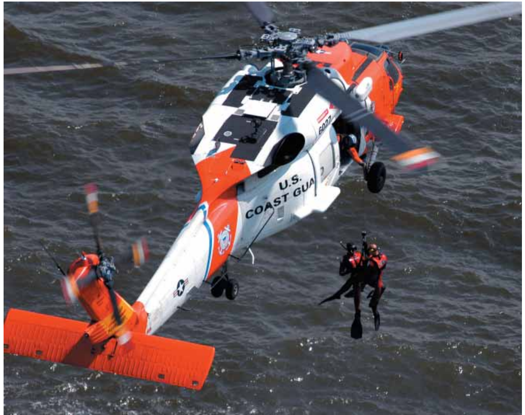
MH-60T No. 6027 conducts a hoist recovery during a training mission following the aircraft’s upgrade. The H-60 Conversion Project will upgrade 42 Jayhawks with state-of-the-market avionics, a new wiring harness and advanced mission systems at the Coast Guard Aviation Repair and Supply Center, Elizabeth City, N.C. USCG photo
