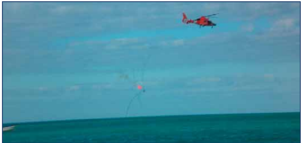
Boat Trap can be deployed from Coast Guard helicopters in flight. Recently, the R&D Center and the Department of Homeland Security's Science and Technology Directorate successfully demonstrated Boat Trap against a 33-foot speed boat powered by twin 200 horsepower motors. U.S. Department of Defense photo
