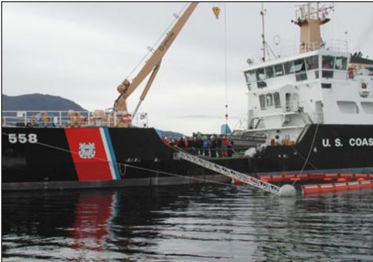
The USCGC Anthony Petit deploys oil spill containment boom during a training exercise in Ketchikan, Alaska.
