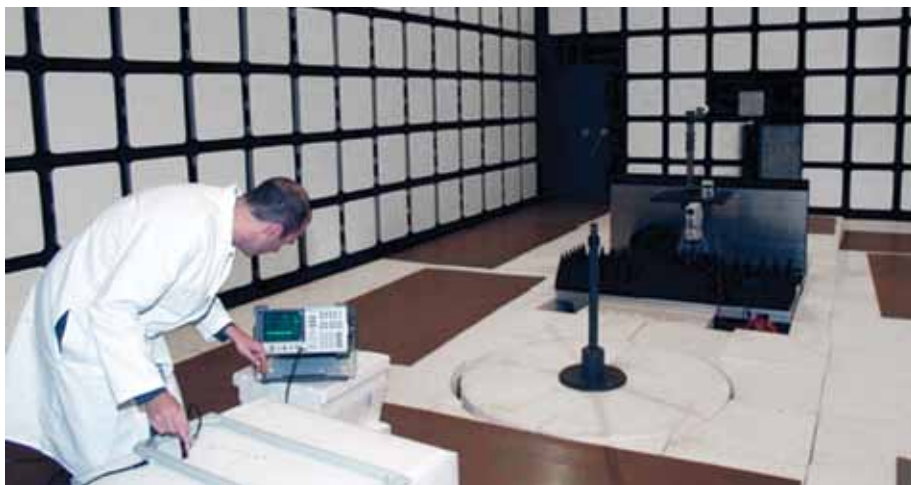
Testing medical implants for susceptibility to radiofrequency interference
