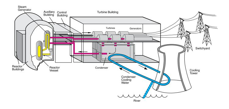
fissionable uranium. Thus, there is not enough fissionable material for an explosion. The illustration above shows how the heat from the fission process is used to make steam and generate electricity at Watts Bar.
