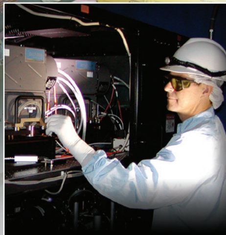
Diagnostics that excel at precision measurements over short timescales and distances are essential to high-energy-density science experiments. Key diagnostics include (above) Dante, a broadband, time-resolved x-ray spectrometer, and (right) VISAR, a time-resolved Doppler velocity camera, which in this photo is being aligned by Livermore scientist Gene Frieders.
