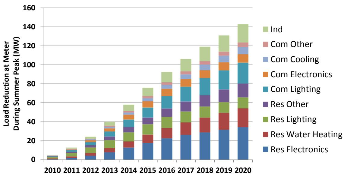
Since the savings shown in the figure from theses measures is estimated at the customer meter, they would provide substantially smaller summer peak flow reductions on the SoA and SoN paths. After adjusting for losses between the meter and the transmission constraints, and applying the 0.37 load flow distribution factor, we estimate that identified energy efficiency measures could reduce flows on SoA and SoN by 57 MW in 2020.
