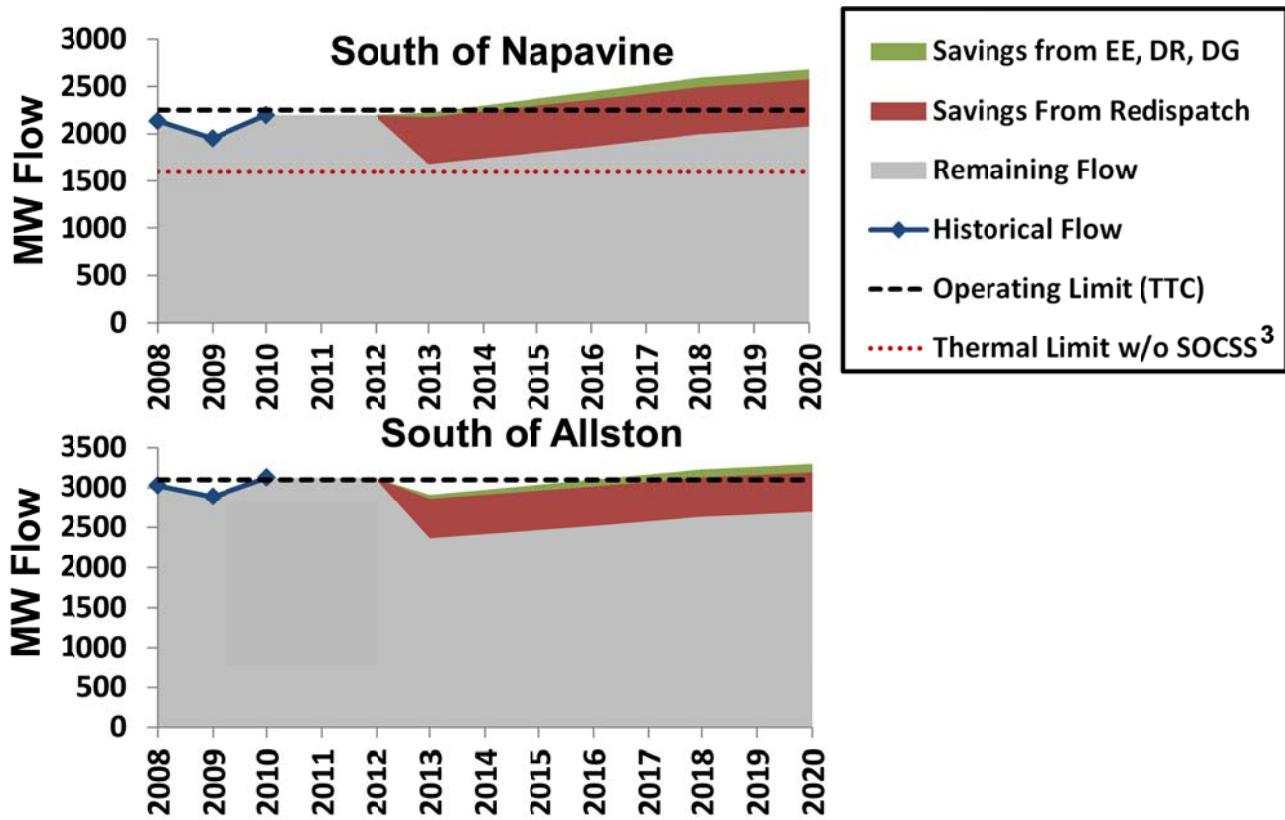
**Figure 2. Identified non-wires potential and resulting flows, Case 1 load forecast.**
