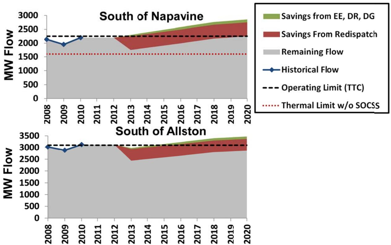
**Figure 3. Identified non-wires potential and resulting flows, using Economic Sensitivity Case load forecast.**
