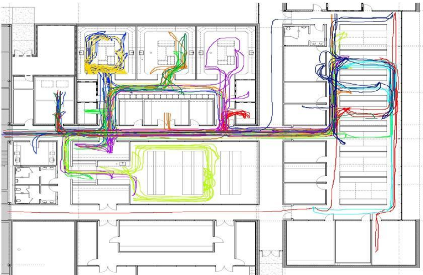
Figure 17: Current state spaghetti chart of a simple sexual assault case. A total of 12,687 feet (2.4 miles) were traveled to complete processing this case. Each different color represents a different step of the process.
