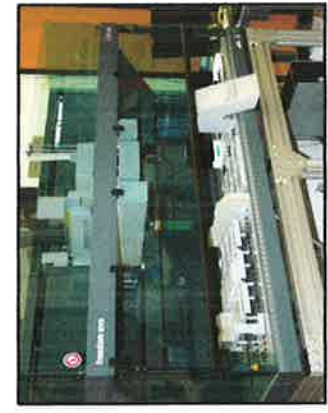
Figure 3. Immediately following DNA extraction, the lysate plate and extraction plate are stored in addition to the sera and blood. The Freedom EVO ® 200 is used to transfer the DNA into the barcoded boxes. This process is automated and efficient.
