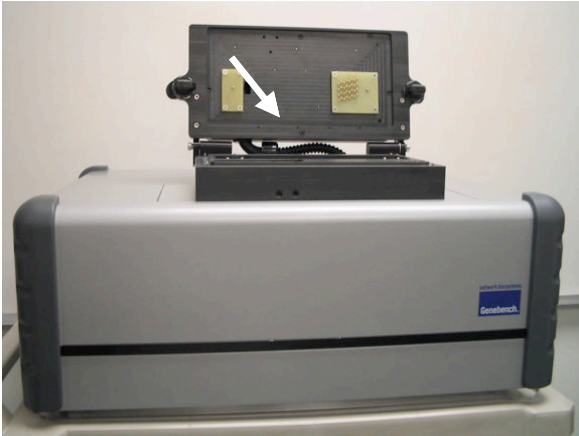
Figure 13. Genebench-FX series 100. Arrow indicates site of microfluidic biochip insertion.
